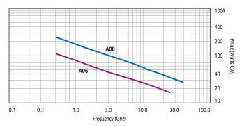
Note: Data at ambient temperature and sea level. Power handling of a cable assembly is also connector dependent and includes variables such as altitude, temperature and system VSWR. See website for connector power handling standards, including altitude, temperature and VSWR derating.
