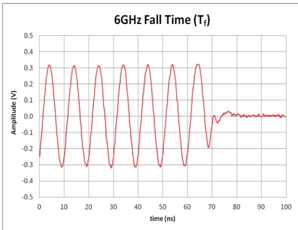
**Figure 4b: Pulse Mod Fall Time,  $f_c = 6\text{GHz}$**
