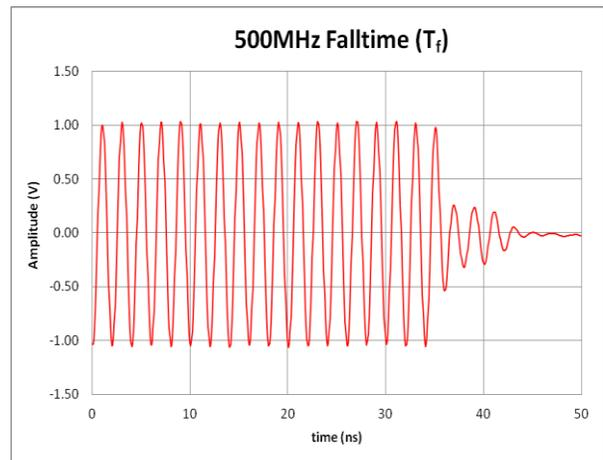
**Figure 2b: Pulse Mod Fall Time,  $f_c = 500\text{MHz}$**
