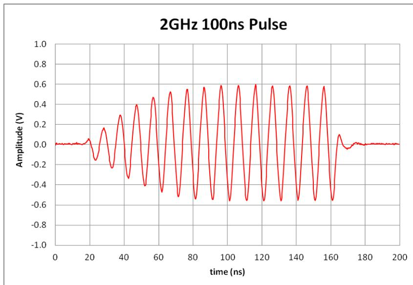
**(Figure 6: Self Pulse Mod  $f_c = 2\text{GHz}$ , 100ns Pulse<sup>2</sup>)**
