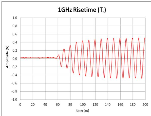
**Figure 2a: Pulse Mod Rise Time,  $f_c = 1\text{GHz}$**
