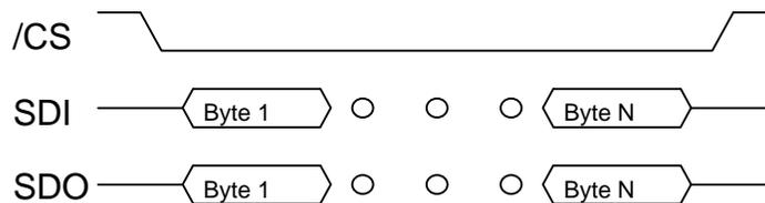
The above figure displays how byte level communications occurs. Any number of bytes may be sent. After /CS goes high, the data is parsed and executed. If no data is sent, the SPI communications module simply resets itself and no parsing or execution of data occurs. If /CS goes high in the middle of a byte transfer (1-7 bits are sent instead of 8) this byte is ignored.
