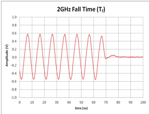
**Figure 3b: Pulse Mod Fall Time,  $f_c = 2\text{GHz}$**
