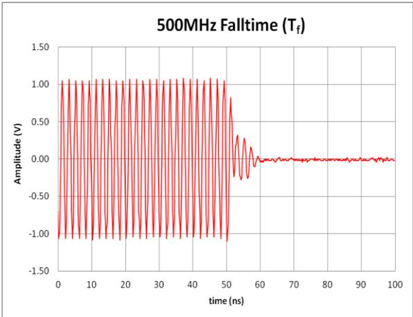
**Figure 1b: Pulse Mod Fall Time,  $f_c = 500\text{MHz}$**
