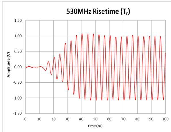
**Figure 3a: Pulse Mod Rise Time,  $f_c = 530\text{MHz}$**
