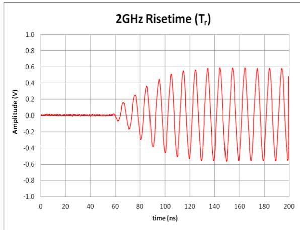
**Figure 3a: Pulse Mod Rise Time,  $f_c = 2\text{GHz}$**
