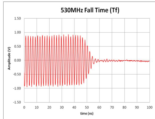
**Figure 3b: Pulse Mod Fall Time,  $f_c = 530\text{MHz}$**
