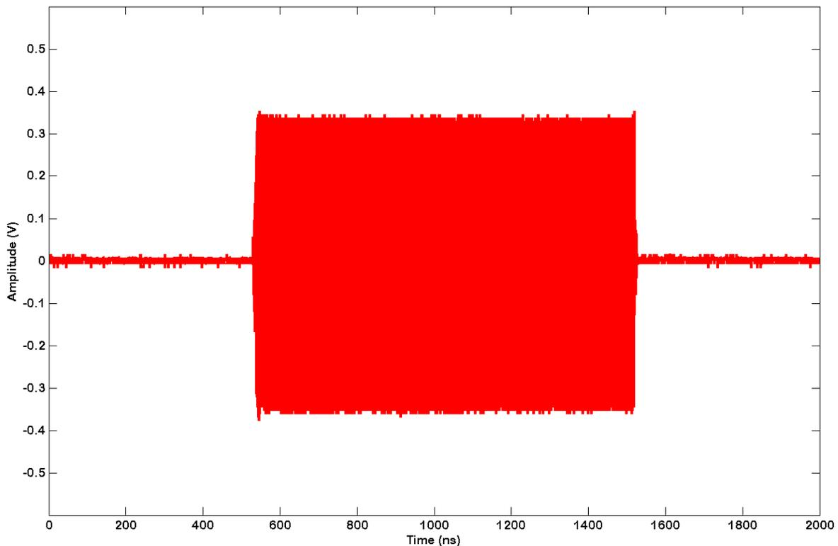
(Figure 1: Self Pulse Mod f<sub>c</sub> = 500MHz, 1us Pulse<sup>2</sup>)
