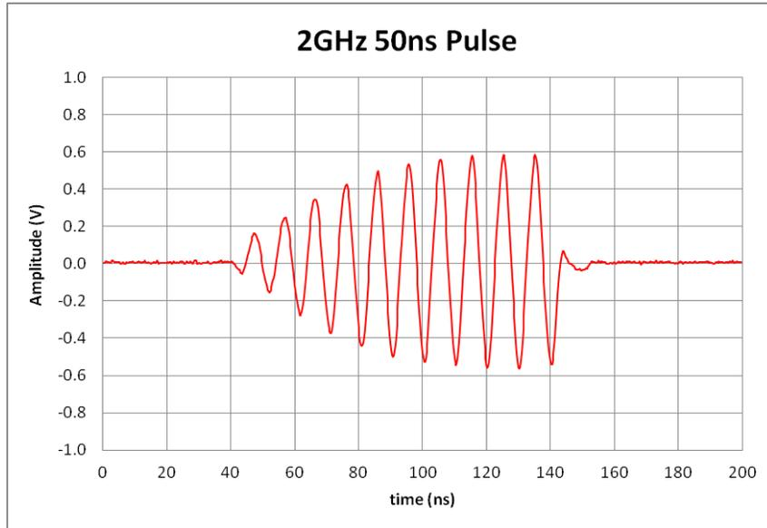
**(Figure 5: Self Pulse Mod  $f_c = 2\text{GHz}$ , 50ns Pulse<sup>2</sup>)**
