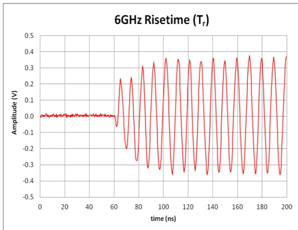
**Figure 4a: Pulse Mod Rise Time,  $f_c = 6\text{GHz}$**
