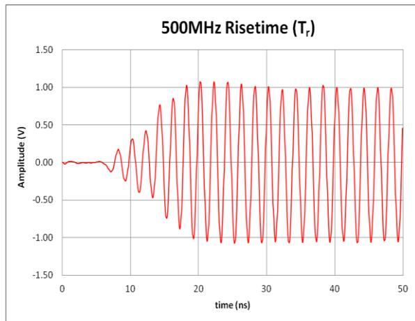
**Figure 2a: Pulse Mod Rise Time,  $f_c = 500\text{MHz}$**
