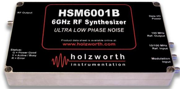
The core architecture of the HSM Series modules is derived from Holzworth’s proprietary NON-PLL design to provide the ultimate in phase / frequency stability. This direct-digital/direct-analog hybrid design was originally developed as a key building block for our phase noise analysis products. The hybrid architecture provides frequency agility & resolution, phase continuous switching and predictable performance without compromising on spurious or phase noise performance.
