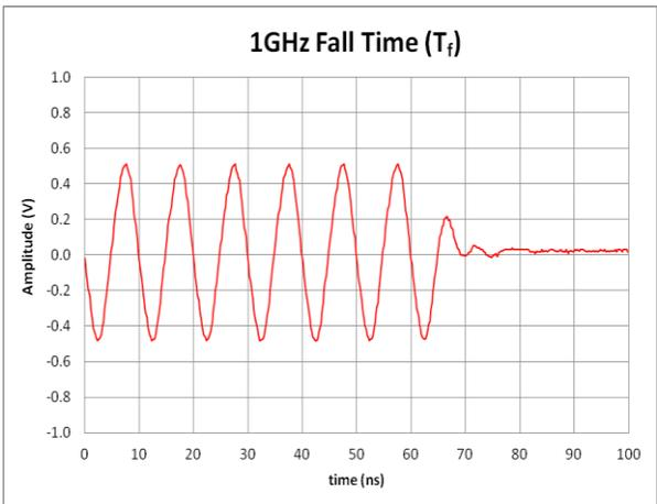
**Figure 2b: Pulse Mod Fall Time,  $f_c = 1\text{GHz}$**
