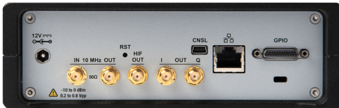
Rear – IF Outputs, 10 MHz Reference, Power, Ethernet
