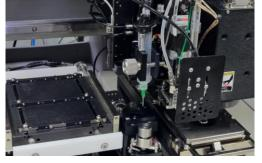
**Heated** applications up to 500°C for different **Eutectic** processes including AuSn, AuGe, AuSi and other interconnection materials.
